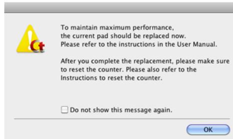
If this message begins to be displayed at startup, purchase an exchange roller kit and replace the worn parts with the consumable parts included in the kit (feed roller and retard roller). For details on the exchange roller kit, see "Exchange roller kit (product code: 5484B001)" on p.113.
